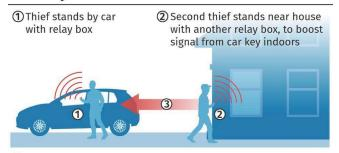
③ Signal is sent back to the box next to car; the car thinks the key is close by and unlocks the vehicle
